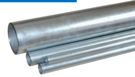
Electrical Metallic Tubing is light gauge steel raceway used to protect wiring from physcial damage and fire. It shields electrical fields emitted by the wiring and acts as a ground. The thick coating of zinc galvanization on the interior and exterior of the conduit provides excellent corrosion resistance from environmental. chemical and mechanical degradation. BBP provides EMT conduit in hex bundles
