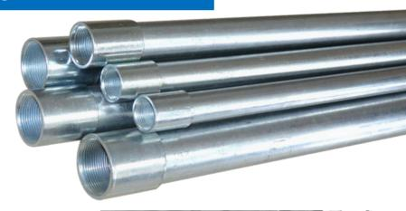
Rigid Metal Conduit is heavy gauge steel raceway used to protect wiring physcial damage and fire. It shields electrical fields emmitted by the wiring and acts as a ground. The thick coating of zinc galvanization on the interior and exterior of the conduit provides excellent corrosion resistance from environmental, chemical and mechanical degradation.
